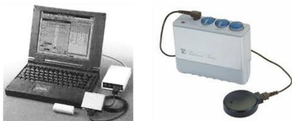
Figure 3: Former Advanced Bionics programming box besides laptop (left; image source: Kessler, D. K. (1999)) and pocket processor (right; image source: Childress, T. (2013, p. 6))
