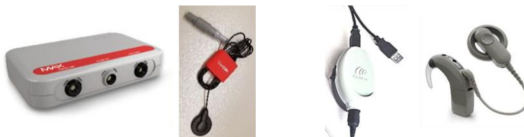
Figure 2: MED-EL programming box and stimulation coil (1 st and 2 nd from left; image sources: MED-EL (2019) and own photography); Cochlear® programming coil and latest eABR compatible speech processor (3 rd and 4 th from left; image sources: CI Shop (2019) and Cochlear (2019))
